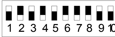
KPS-101 DIP Switches – On/Up, Off/Down – Example: Zone 6, System 1, IR ‘Off’, Termination ‘On’
